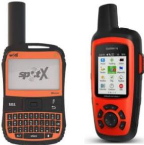
As of 2019, SEND devices can be either one-way transmission devices, such as the basic SPOT, or two-way satellite transmission units such as the Spot X or Garmin in-Reach units.
